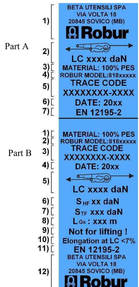
The blue colour of the label immediately identifies the material the strap is made of, namely 100% PES (polyester).
