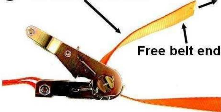
**6** Operate the lever ratchet for tensioning of the belt
